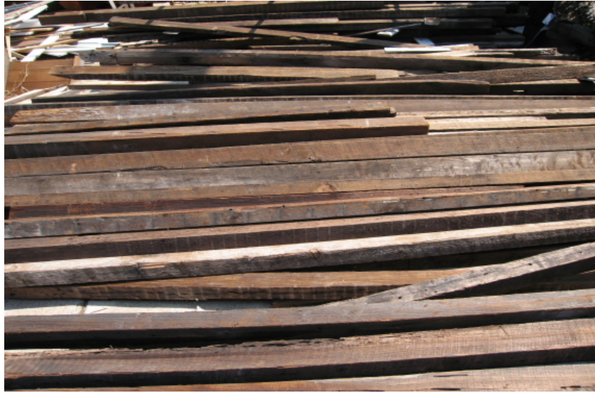
Figure 3. Reclaimed cypress and pine lumber from New Orleans homes.
